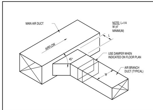
**A** RECT. DUCT CONNECTION DETAIL NO SCALE
